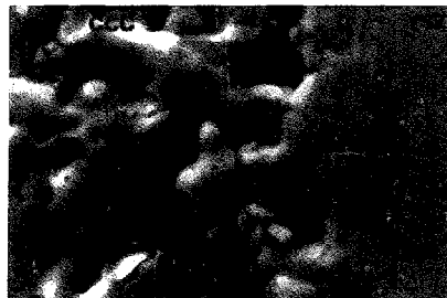
Fig. 17. SEM micrograph showing a cross section of an electrode without a P-layer (K320, series 2).
